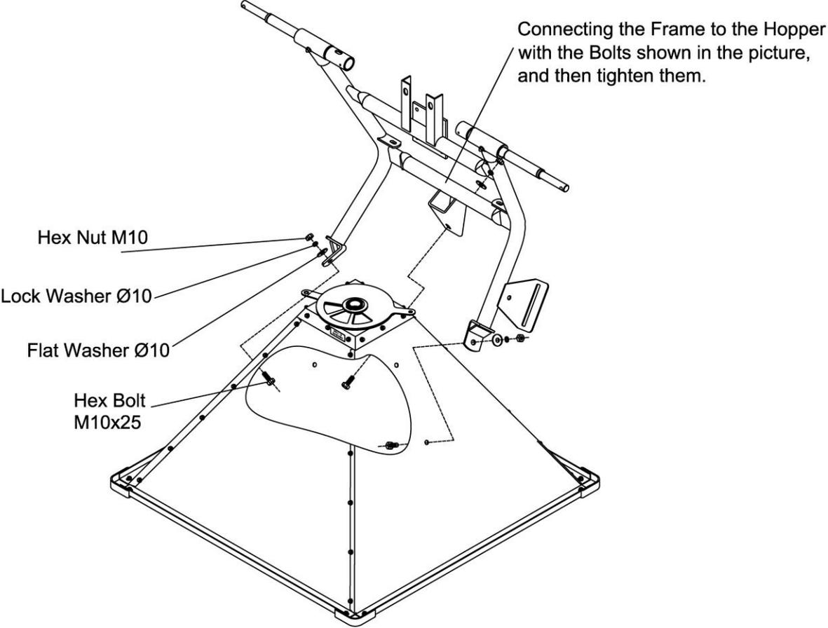
When assembly, please have the hopper side lay, the hopper panel with label should be put in downwards.
