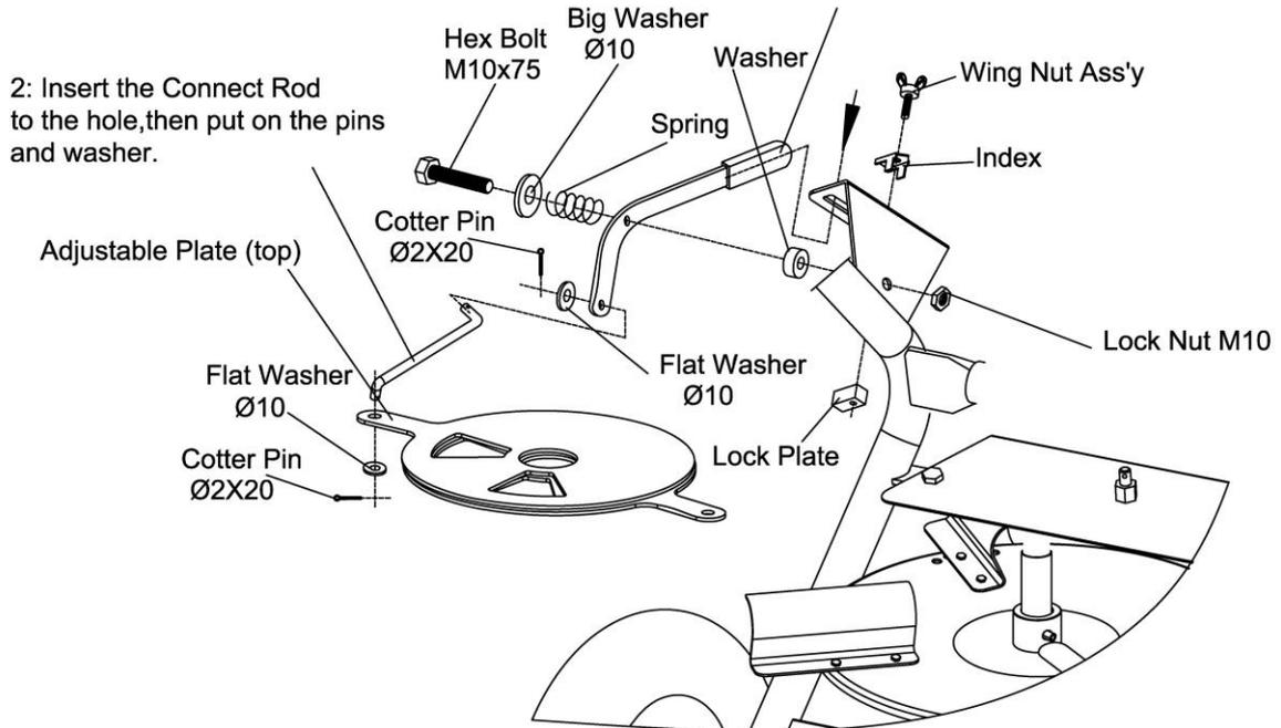
Moving this handle, it could adjust the stuff volume that spreader out on the bottom.
