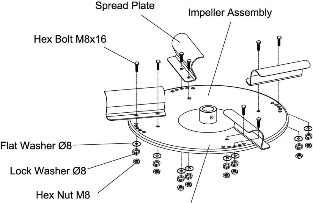
Assemble the Spread Plate to the Impeller accordingly, secure with bolts, washers & nuts.
