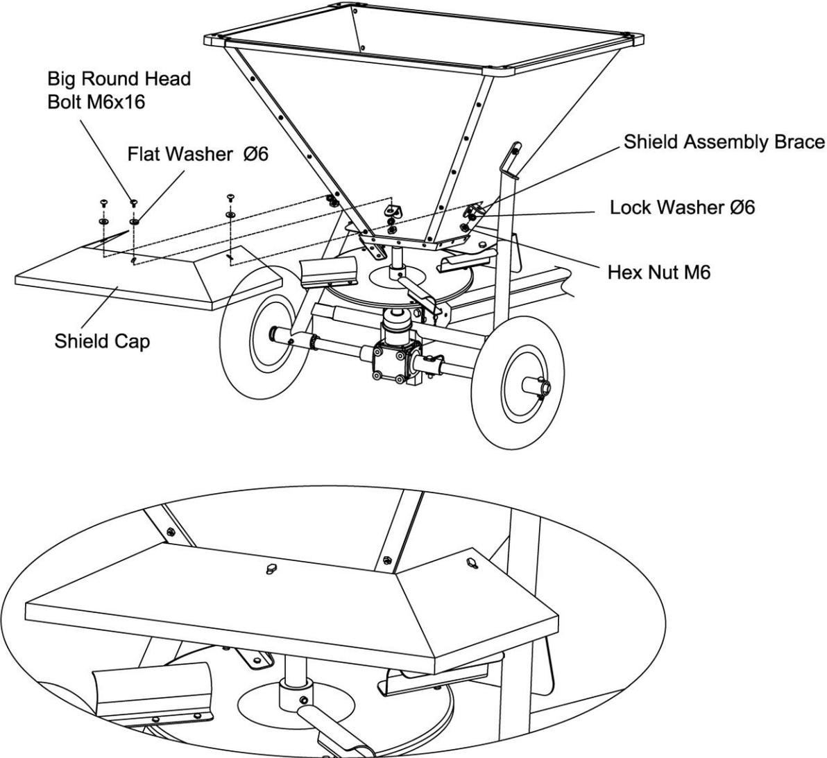
Tighten all bolts as well as the bolts that haven't tightened in the above step.
