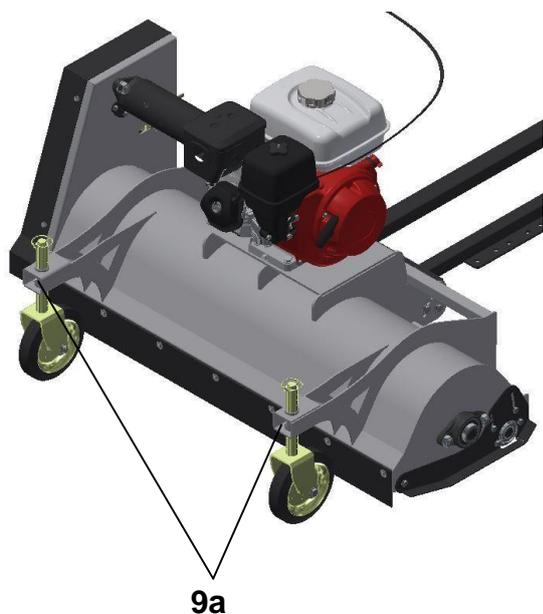
**Obr. 9:** Greasing points
