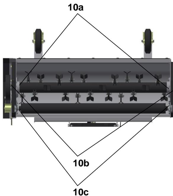
**Obr. 10:** Greasing points
